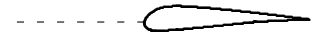
A static airfoil in an airstream coming in horizontally from the left. The shown streamline (dashed) ends in the forward stagnation point.
