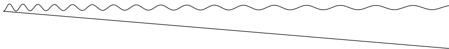
Figure 22.4: Gravity waves coming in from the right towards a coast along a gently sloping flat bottom. The waves increase gently in amplitude as they decrease in wavelength. When the amplitude becomes comparable to the depth (on the left), non-linear effects take over and make the waves break.
