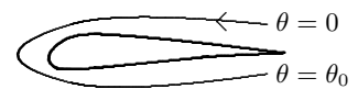
The airfoil outline may be parameterized with a parameter \theta running over the interval 0 \leq \theta \leq 2\pi .
